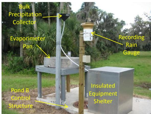
a. Equipment shelter and meteorological equipment placed on top of Pond B water control structure
