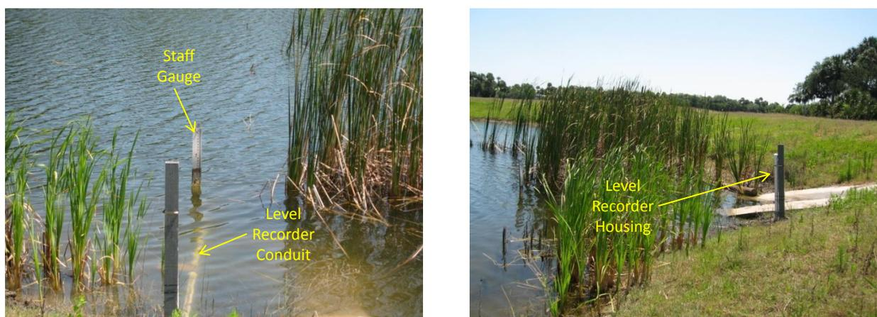
Figure 2-11. Photographs of Staff Gauge and Water Level Recorder Used in Pond B.
