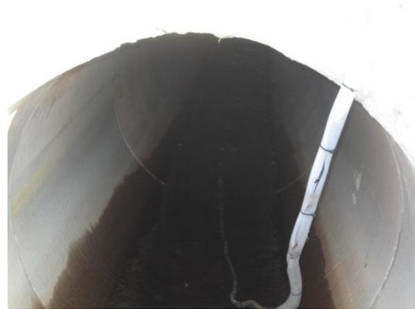
d. Sample tubing and flow probe extended approximately 10 ft into culverts
